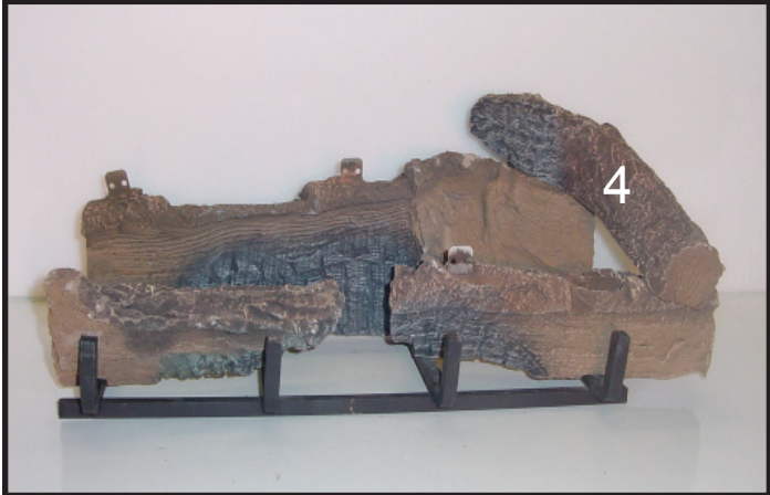
LOG #4 (SRV2045-703): Place log #4 on top of log #1 and log #2 so that the cutouts on the bottom of log #4 fit on the tab on log #1 and will fit in the flat spot on log #2.
